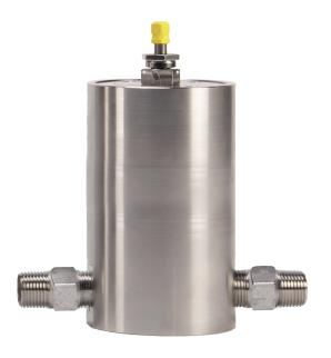
**PTFE Tough** Now available on all models from 2,000 to 15,000 psi, Blacoh's unique PTFE bellows have an excellent flex life, are compatible with virtually all chemicals and solvents, and can withstand temperatures up to 220°F (104°C).
