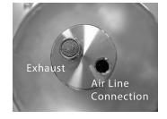
Compressed air should be applied to the dampener charge port at all times for proper operation. In case the compressed air supply to the dampener is interrupted, it is recommended that a check valve be added to the compressed air supply line after the air regulator to prevent the charge from escaping through the air inlet while the dampener is depressurized.
