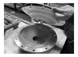
6. The PTFE diaphragm and backup diaphragm are attached to the air control shaft with an anti-extrusion button. Gently pull down on the diaphragms to slide the entire assembly out from the automatic valve in the non-wetted housing and discard the assembly. Take necessary precautions not to scratch or otherwise damage the assembly shaft or the automatic valve when removing the assembly, otherwise, the automatic valve may not function properly.
