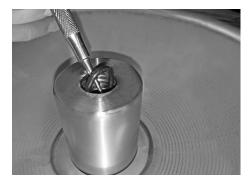
4. Apply a thin coat of lubricant (such as Molykote<sup>®</sup> 55 or equivalent) to new O-rings. In the automatic valve **top** housing, install new -208 O-ring in groove 1, new -114 O-ring in groove 2, and new -019 O-ring in groove 3 (Figure 2). In the automatic valve **bottom** housing, install new -114 O-rings in grooves 4, 5 and 6. The automatic valve will not operate if the O-rings are installed in the wrong grooves (Figure 2).
