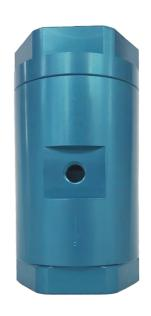
SENTINEL Normally Closed Shutoff Valves offer an excellent high flow coefficient and a low pressure drop that equates to overall faster and smoother fluid flow. Valves are pneumatically controlled and use an internal piston to allow or prevent air or fluid flow. The normally closed valve opens when air pressure is applied to the pneumatic control port.
