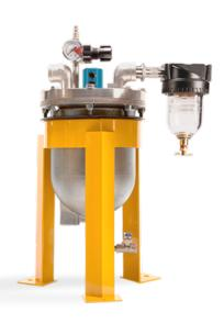
The fully pneumatic SPILLSTOP system attaches directly to the exhaust of an AODD pump. When the pump fails, SPILLSTOP safely captures leaked product and automatically shuts down failed pumps to avoid costly product loss and prevent hazardous spills. Optional warning alarm and backup pump switchover further minimize system downtime for maximum productivity.
